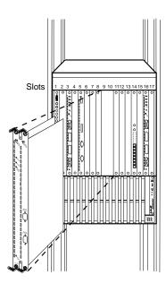
Figure 2-1. Installing the 6416SW Module in an ONcore Hub
